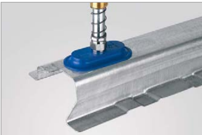
Flat suction cups SAOF being used for handling pressed sheet-metal parts
