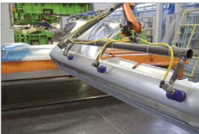
Bellows suction cups SAOB being used for handling car bodywork components
