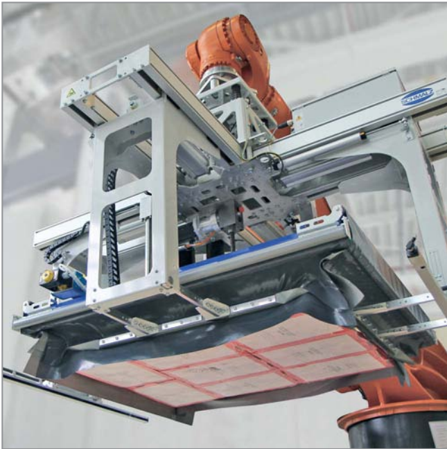
Function tests on a vacuum layer gripping system in the company's own testing laboratory
