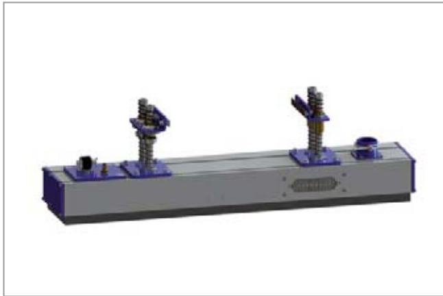
Mounting example spring plungers FST-STARR/FLEX
