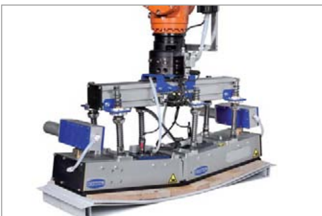
Mounting example spring plungers FST-FLEX
