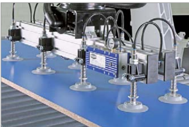
Mounting example spring plungers FSTF
