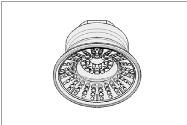
System design bellows suction cup SAB HT1 (1.5 folds)
