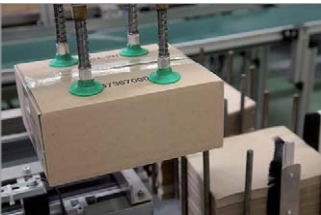
Bellows suction cups SPB1 being used for handling of cardboard
