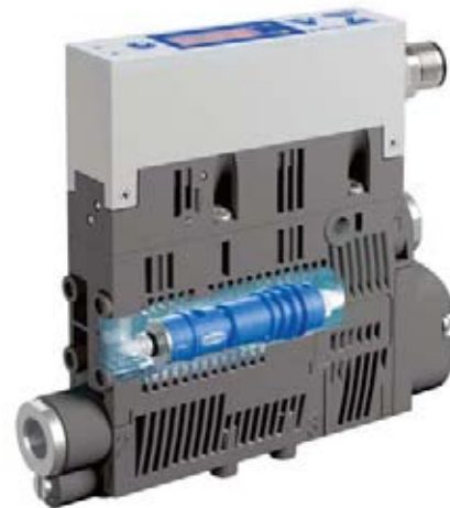
Ejector core with eco nozzle technology and integrated automatic air-saving function
