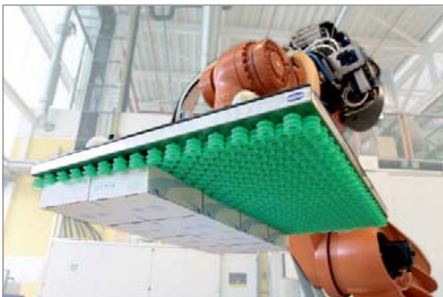
Bellows suction cups SPB2 P being used for handling of cardboard boxes
