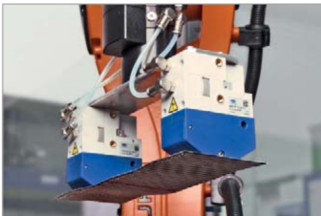
Needle grippers SNG-AP being used for handling composite textiles
