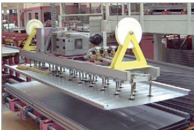
Flat suction cups PFYN VU1 being used for handling large sheet metal parts
