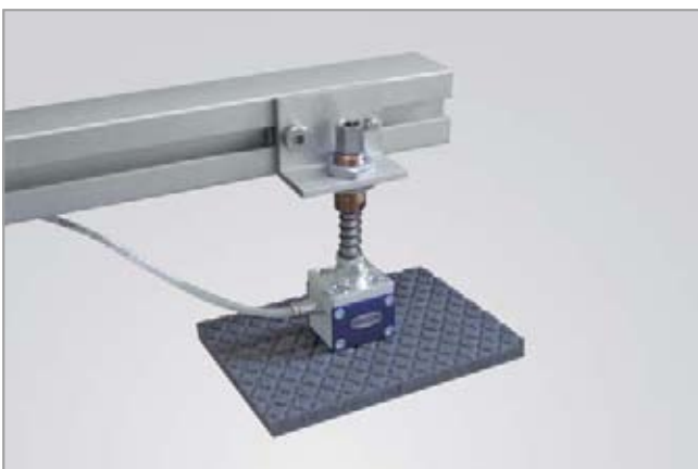
Needle grippers SNG-M being used for handling structured foam materials
