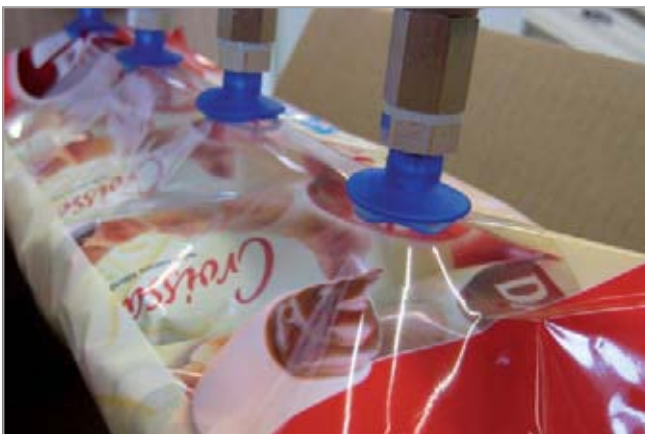
Bellows suction cups FGA PVC being used for handling non-rigid workpieces
