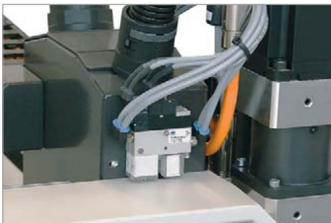
Central vacuum generation by compact ejectors SCPM
