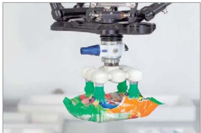
The vacuum end effector with bellows suction cups SPB4f handling pouches with strong wrinkling and low filling degree
