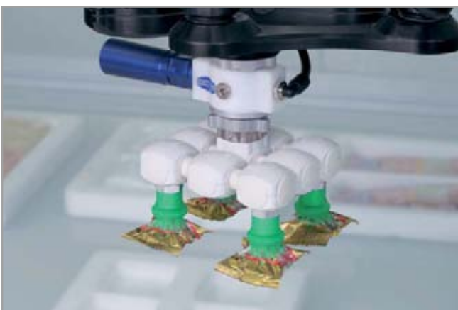
Bellows suction cup SPB2f for handling bags
